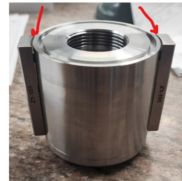
Z1 Heat Source and Shielding Capsule
